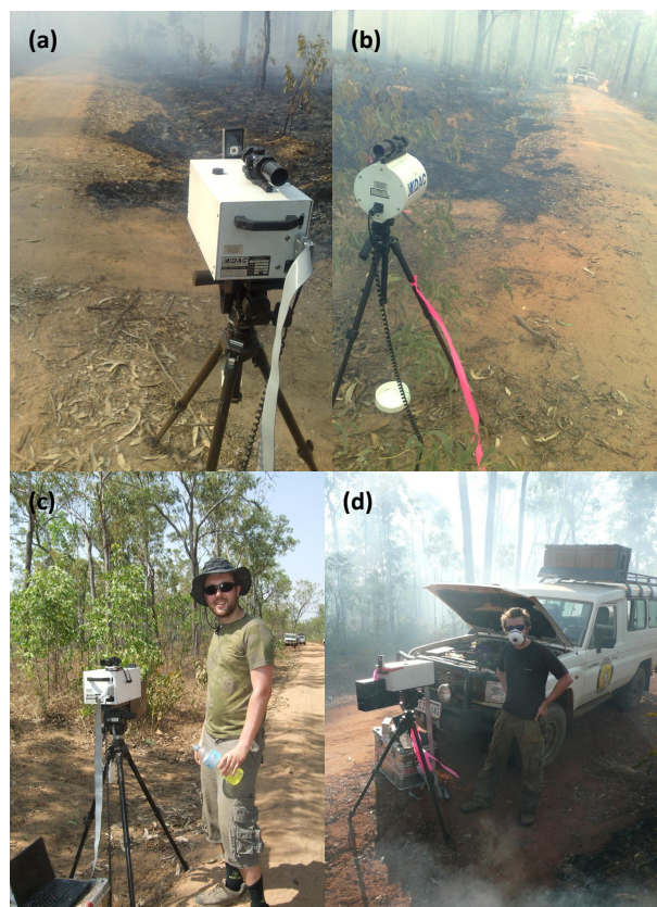
Figure 7.8: The FTIR spectrometer set up beside the burn plots ((a), (c) and (d)) of the Australian field campaign. The IR lamp was positioned approximately 40 m away such that during the fires the smoke plume was able to pass between the two instruments (b). A car battery was used to power the spectrometer for some fires (d), otherwise a motorcycle battery was used. Images taken by author.
