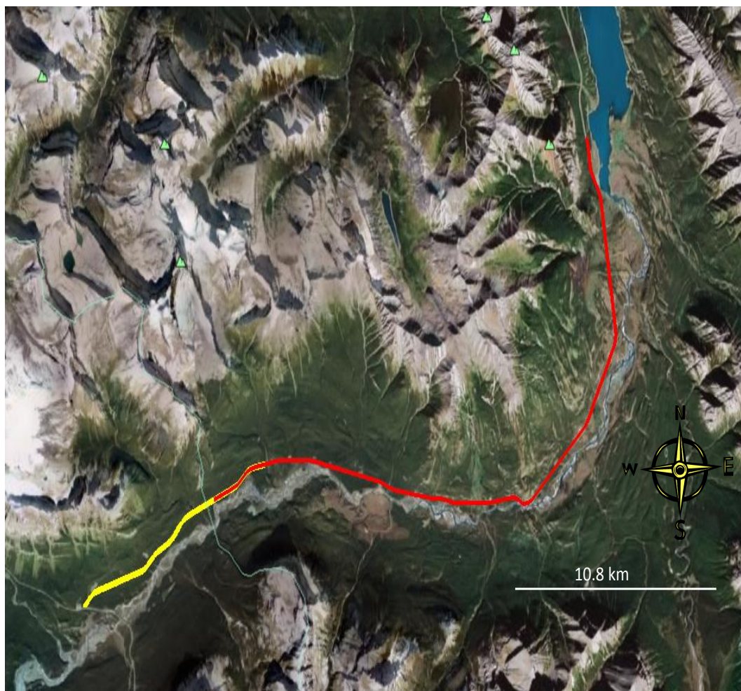
Figure 5.13: The traverses of the DOAS vehicle of fires CF1 (red) and CF2 (yellow), taken from GPS data measured in the vehicle. The traverses of fire CF1 are much larger than those of fire CF2 due to the larger plume of CF1, resulting in more distance to travel to enter clear sky. Background images are taken from Google Earth.
