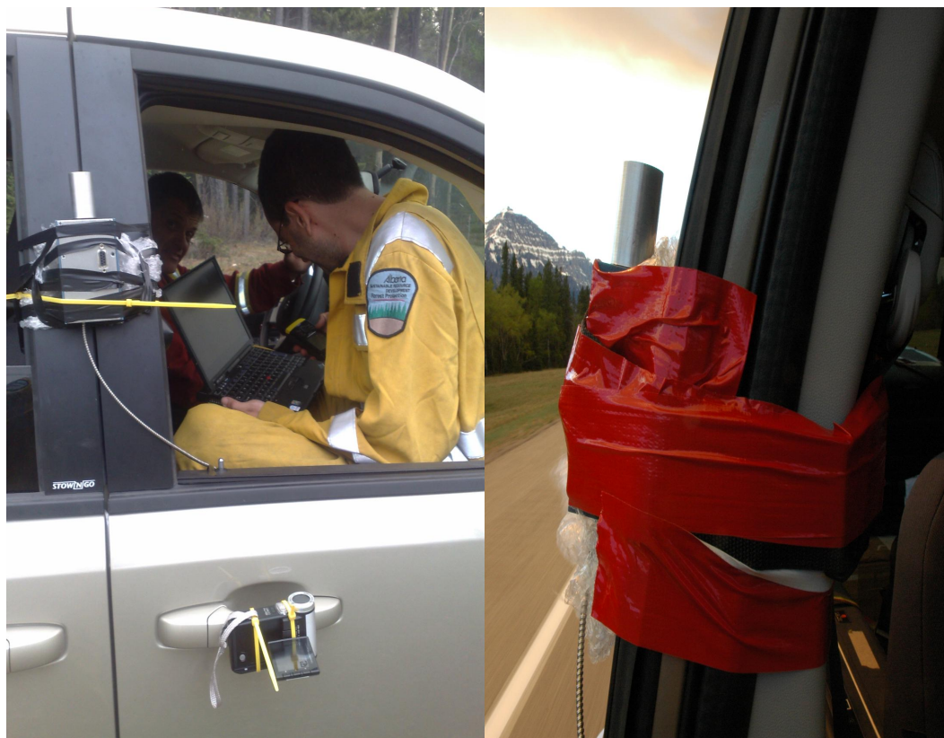
Figure 5.9: The set up of the DOAS during data collection, with the telescope mounted on the outside of the car and pointing to zenith, connected to the spectrometer inside the car via an optical fibre. The connecting laptop is also kept inside the car. Photos taken during the Canadian field campaign.
