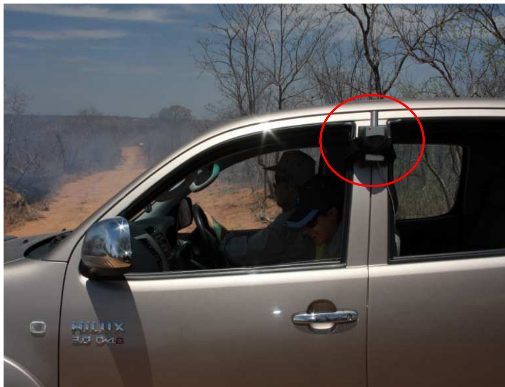
Figure 5.8: Photograph showing how the UV DOAS telescope was positioned on the car during the traverses. Note the optical fiber connecting to the spectrometer inside the car. Photo from the South African field campaign
