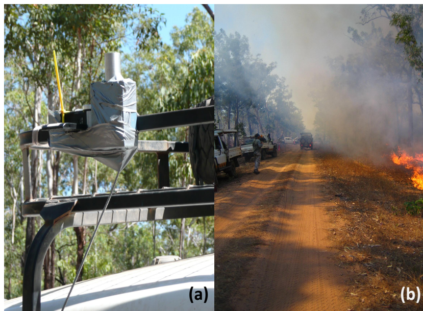
Figure 7.7: The telescope of the UV-DOAS spectrometer attached to the vehicle pointing zenith for one of the fires of the Australian field campaign a). The vehicle then traversed back and forth during the fire, perpendicular to the direction of travel of the smoke plume, as shown in b). Images taken by author.
