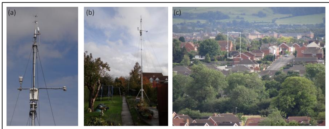
Figure 2-7 Eddy covariance station and meteorological measurements situated in the garden of a residential property.
