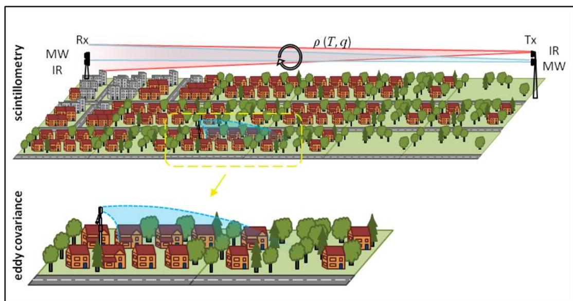
Figure 1-1 A schematic representation (not to scale) of the scintillometry technique: infrared (IR) and millimetre-wave (MW) beams propagate from transmitter (Tx) to receiver (Rx) refracted by turbulent eddies of density \rho at temperature T and humidity q ; and the eddy covariance technique.
