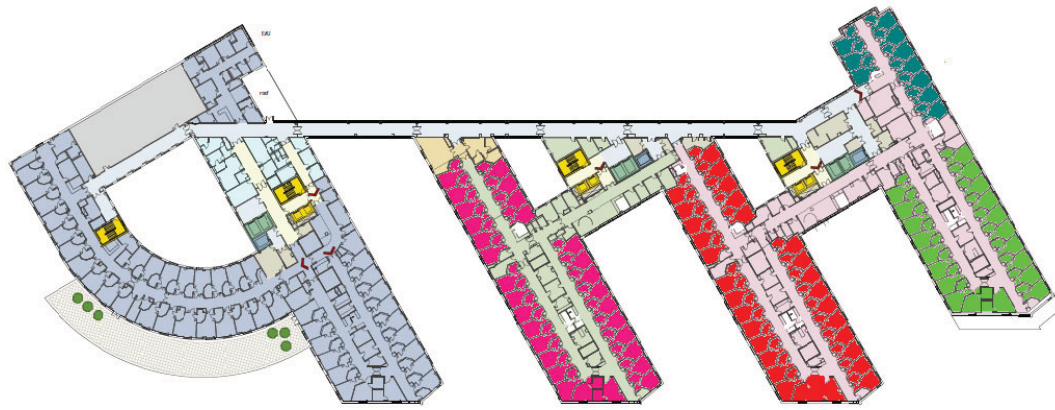
FIGURE 2 Floor plan showing 'perimeter' design of new hospital with single rooms wrapped round the outside of each ward 'finger' and ward support facilities down the centre. Reproduced with kind permission from Stantec.
