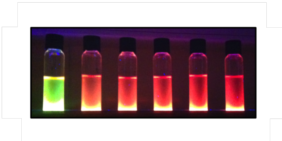
Figure 3.2: Aliquots of CdZnSeS alloyed QDs in hexane taken after injection of the selenium/sulphur precursor solution at time points of 30 sec, 1 min, and every min thereafter (vials arranged left to right).
