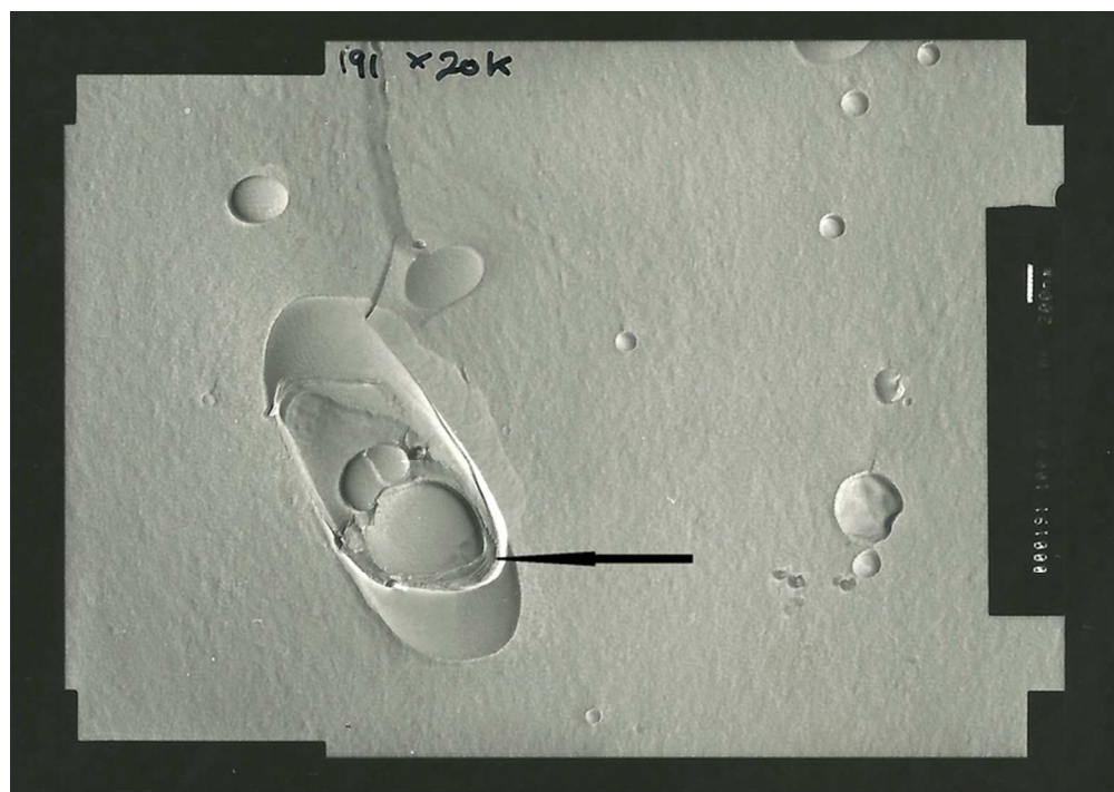
31 32 33 34 35 36 37 38 39 40 41 42 43 44 45 46 47 48 49 50 51 52 53 54 55 56 57 58 59 60 Figure 7. Freeze-fracture electron micrographs of dispersions of equimolar mixtures of distearoylphosphatidylcholine and cholesterol in A. 20% w/w propylene glycol, B. 60% w/w propylene glycol and C. 100% w/w propylene glycol. In micrograph A, the arrow indicates the appearance of a lamellar stack. In each micrograph, the scale bar represents 200 nm. 69x48mm (300 x 300 DPI)
