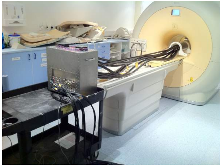
Fig. 4.5 PET-MR experimental setup with the PANDA II insert, the Philips Achieva 3T scanner and the rotational phantom, driven by a 3.5 m carbon fibre rod. (Soultanidis et al. (2011), © IEEE 2011)
