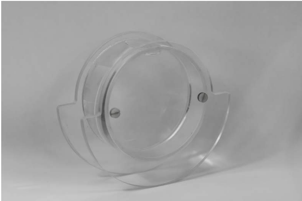
Fig. 5.7 Homogeneous phantom for normalization scan
