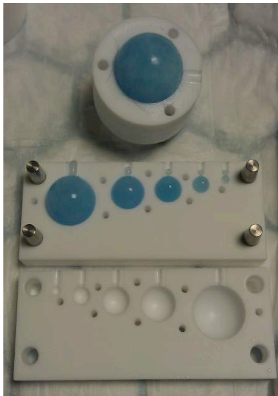
Fig. 3.9 The PVA cryogel moulds. The sphere diameters are: 5 mm, 10 mm, 15 mm, 20 mm, 30 mm and 40 mm
