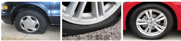
(a) Tire is flat. (b) Tire is under-inflated. (c) Tire is OK.
