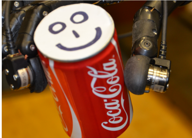
FIGURE 2.5: Intrinsic force-torque sensor with soft rubber layer
