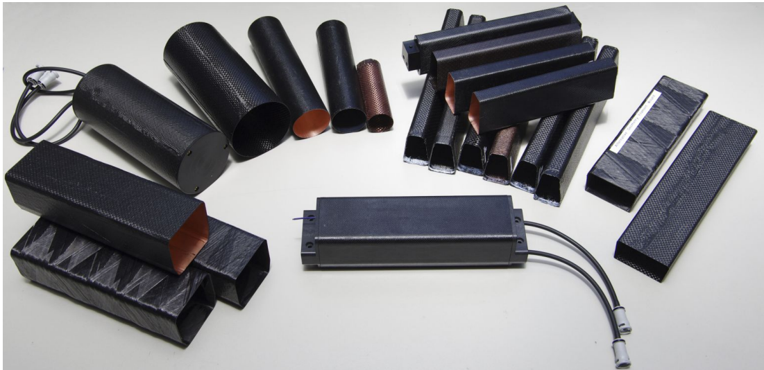
Figure 4.2 Overview of carbon fibre composite housings produced during the Hyperion II D development. Various mandrels target the specific geometric requirements of different housing approaches. In addition to pure carbon fibre fabrics, multiple laminates were fabricated with alternative materials, e.g. fibre glass, metal layers and coated fibres. Furthermore, the feasibility of carbon fibre winding was demonstrated.
