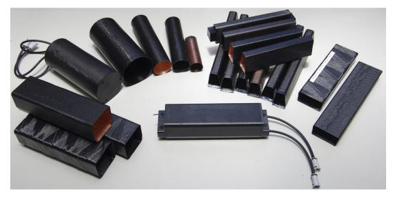
**Figure 4.2** Overview of carbon fibre composite housings produced during the Hyperion II<sup>D</sup> development. Various mandrels target the specific geometric requirements of different housing approaches. In addition to pure carbon fibre fabrics, multiple laminates were fabricated with alternative materials, e.g. fibre glass, metal layers and coated fibres. Furthermore, the feasibility of carbon fibre winding was demonstrated.
