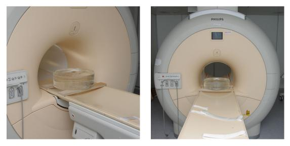
**Figure 3.6** Setup to measure  $B_0$  distortion maps. Test objects are placed centred on an oil filled MRI phantom.
