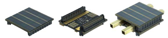
**Figure 3.1** MRI-compatible digital SiPM sensor tile, interface board and assembled detector stack with cooling pipes. The edge length of the quadratic sensor tile is 32.7 mm.
