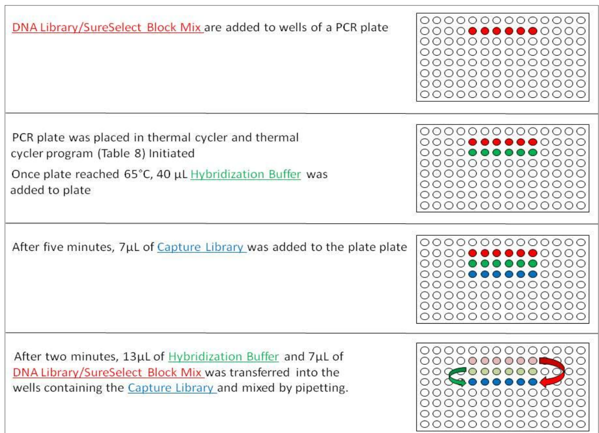
Figure 18 PCR Plate Setup for SureSelect Hybridization. Reagents and the wells to which they should be added in a 96 well plate are colour-coded.
