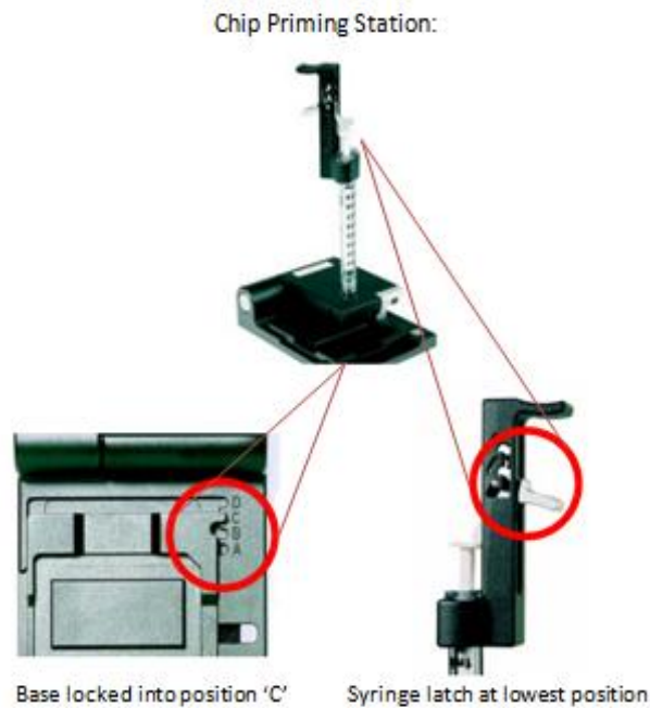
Figure 10: Setting up the Chip Priming Station. Figure modified from images in the Agilent DNA 1000 Kit Quickstart Guide G2938-90015 (for URL, see appendix 2)
