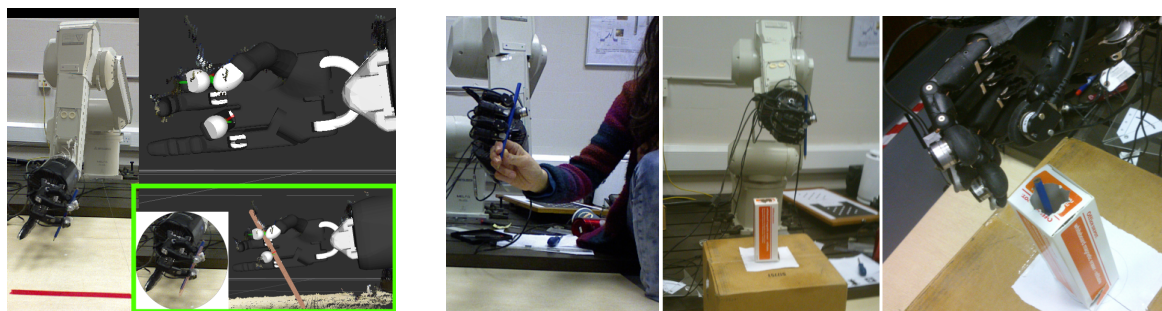
(a) Clockwise from left: Robot grasping the pencil; Point cloud overlaid with the robot model; Result of the pose estimation
