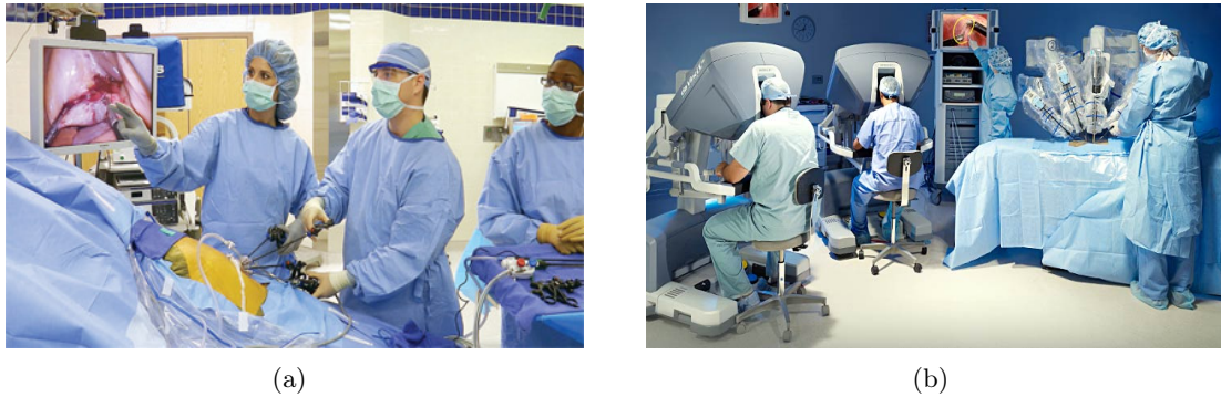
FIGURE 2.3: Surgical Theatre for: (a) Conventional Endoscopic Surgery (CES) in which the surgeon manipulates the surgical instruments using his hands and (b) Robotic-assisted Minimally Invasive Surgery (RMIS) in which the surgeon operates remotely moving the robots from a console.
