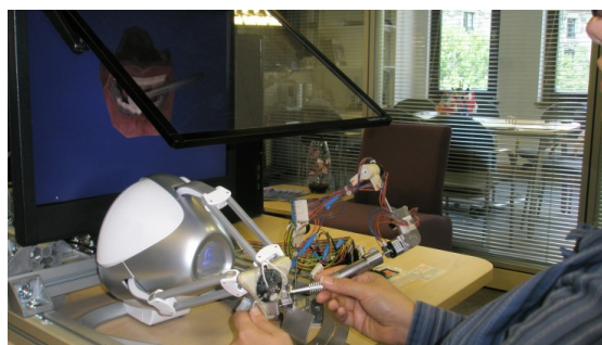
FIGURE 2.5: Haptic user interface: Geomagic Touch Haptic Device and Virtual Reality Simulator.
