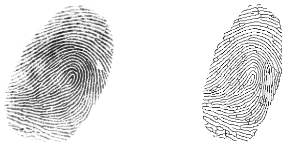
Fig. 4.5 Before and after performing the thinning preprocessing step on the fingerprint images
