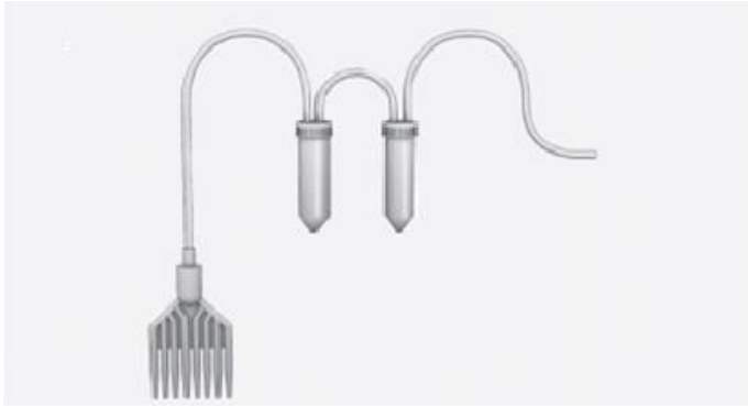
Figure 2.1: Assembled set-up for vacuum assisted emulsion breaking and bead recovery (Reference: Roche emPCR method protocol).
