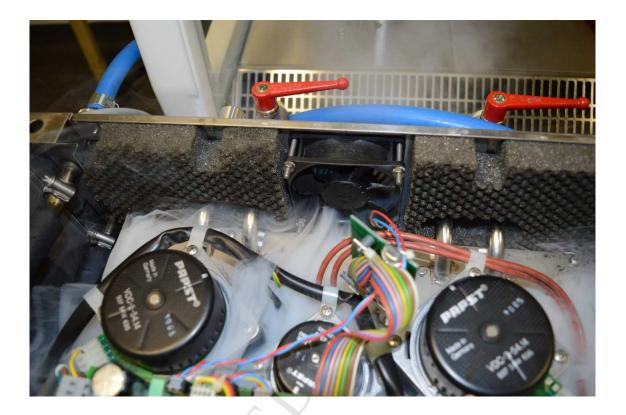
Figure 4b. Video of smoke pen to visualise air flow path as it is pulled away from the pumps and gaps associated with the water tanks to the rear fan and as it is excited from the HCU.
