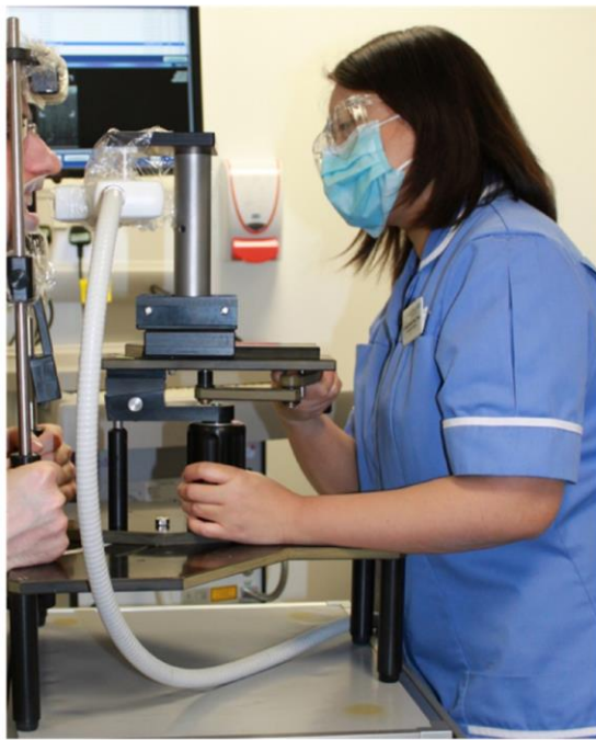
Figure 2 Clinical Optical Coherence Tomography imaging set up: Clinical OCT Probe mounted in geometry stabilizing unit for in vivo imaging of four 1 mm x 1 mm x 1.5 mm (x, y, z) volumes from of the labial aspect of each of the maxillary incisors in order to acquire B-scan stacks. Example of resulting single B-scan (x,z) from which 250 individual A-Scans were extracted for analysis using a custom designed algorithm, designed to quantify the back scattered OCT signal intensity from the superficial subsurface enamel (D).
