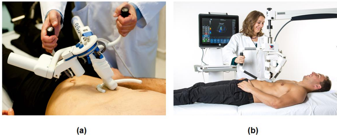
Fig. 2.1. Example uses of the tele-operated robotic systems on patients from the projects funded by ESA: (a) the robot from the ARTIS project which focused on light weight. (b) TESSA project, which resulted in the commercial robot MELODY. Figure reproduced from [136].
