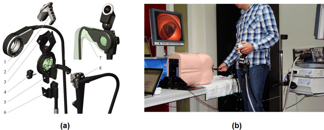
Fig. 2.10. (a) Exploded view of the coupling mechanism: (1) Drive unit, (2) Remote control, (3) Holder remote control, (4) Plug, (5) Sterile interface, (6) Docking station, (7) Sterile bag, (8) Endoscope. (b) Phantom experimental setup showing the control of the robotic NOTES endoscope. Figure reproduced from [182].
