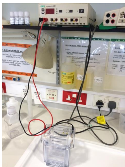
Figure 20: Illustration of SDS electrophoresis setup
