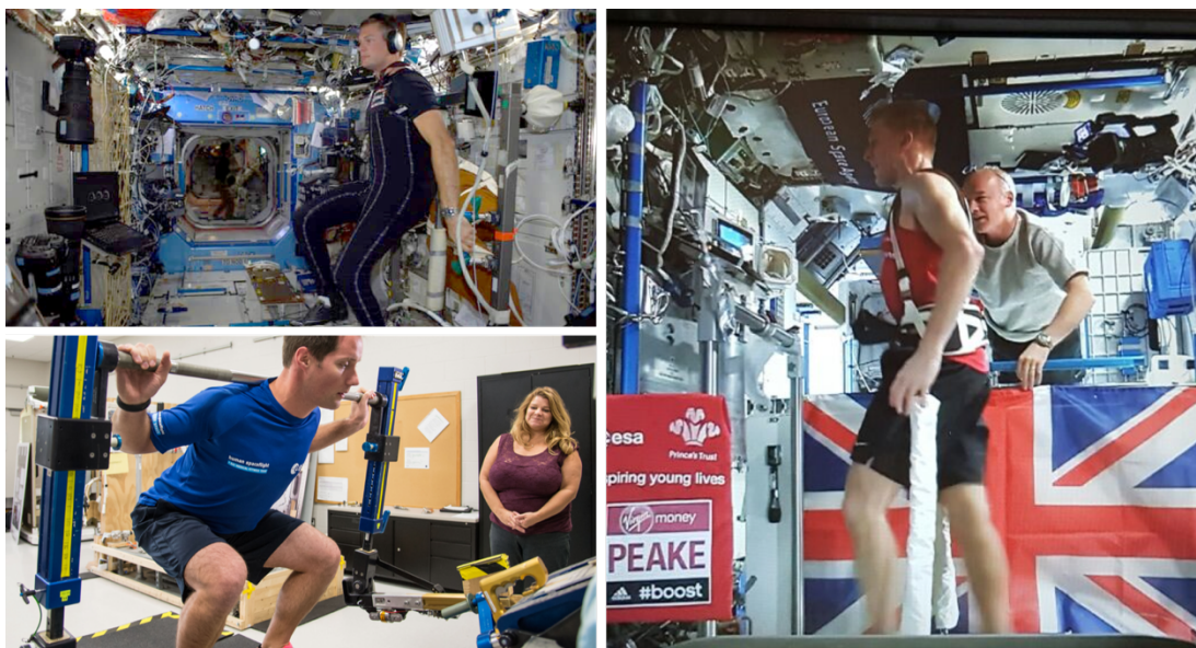
Figure 5. Exercise Countermeasures currently on use on the International Space Station including cycling on CEVIS (top left), resistance exercise on ARED (bottom left) and treadmill running on COLBERT (right). Image Credit ESA and NASA.
