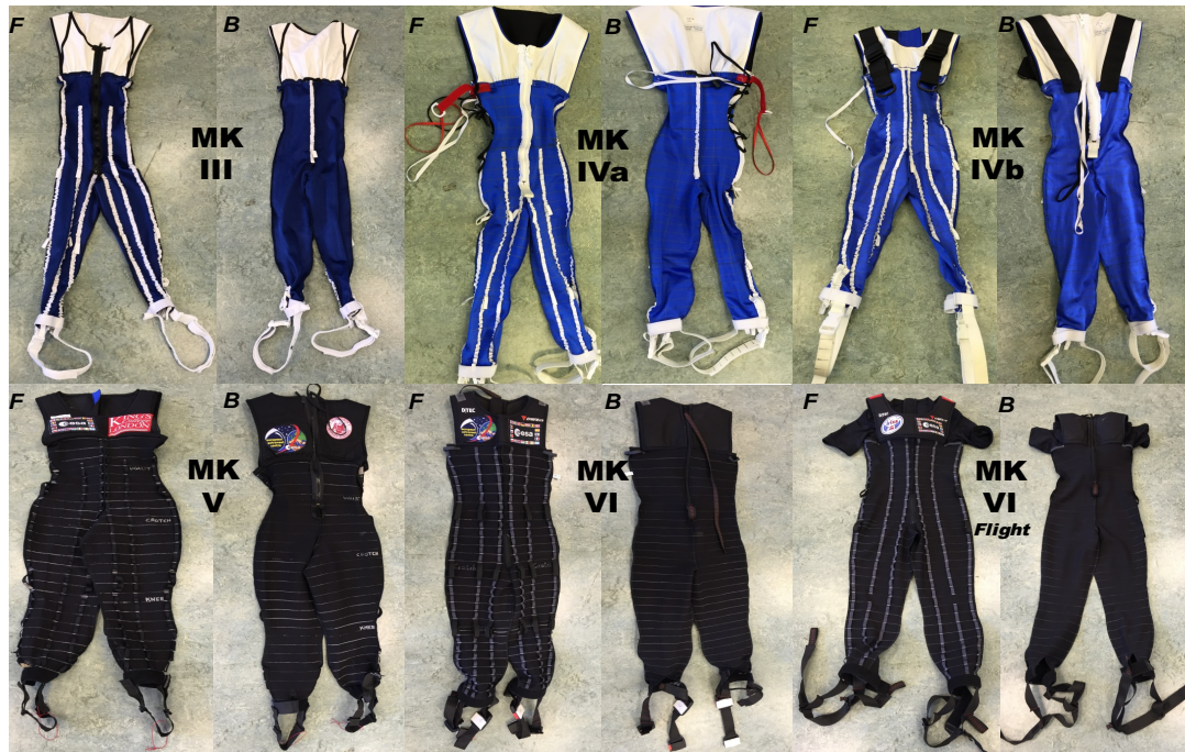
Figure 7. Evolution of the European Space Agency's SkinSuit to current Mk VI flight model. Image credit – European Space Agency and King's College London.
