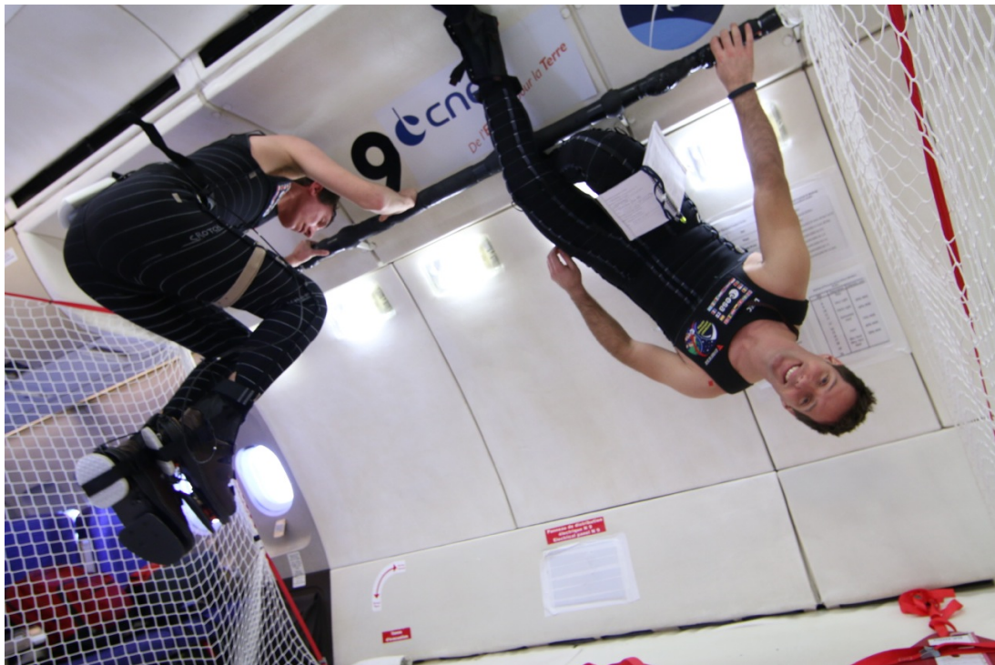
Figure 12. Experimental testing of the Mk V SkinSuit during parabolic flight with ESA Astronaut Thomas Pesquet, performed to optimise design and characterise SkinSuit loading and comfort, prior to long duration (8h) ground model testing and spaceflight operational testing. Image Credit: ESA.
