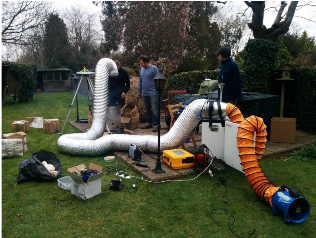
Figure 4.9: Deployment of Partisol Sequential Air Sampler, smoke sampling box and LGR analyser in crop residue bonfire tests, designed primarily to provide a DustTrak calibration for this type of smoke.
