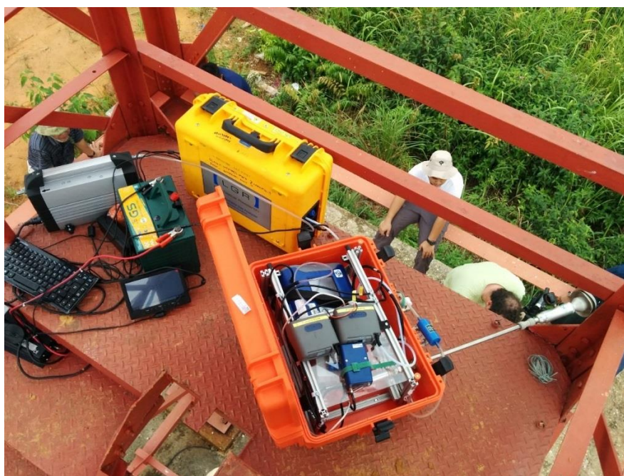
Figure 4.6: Deployment of updated smoke sampling system in the field, including two main parts, LGR ultra-portable greenhouse gas analyser which provided CO 2 , CO, CH 4 and H 2 O measurements (closed yellow box at top) and the new smoke sampling box which provided CO 2 , CO, PM 2.5 and BC measurements (opened orange box in the middle).
