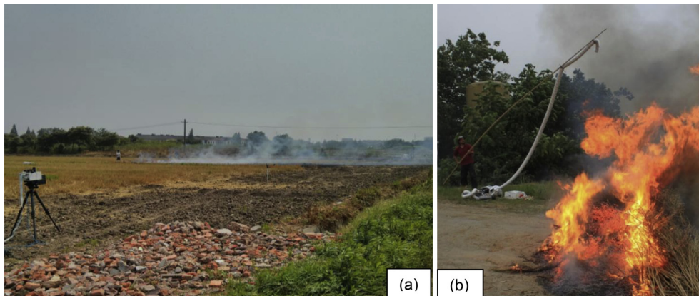
Fig. 3. Photographs of two of the agricultural fires studied herein. (a) was taken during Fire No. 4, which is a spreading wheat stubble fire. The wind was blowing from west to the east (left to right in the photo), the smoke sampling box is standing downwind inside the ground level smoke plume, whilst the FTIR spectrometer was located north of the fire viewing southward to measure the spectra of the IR lamp that was behind the smoke plume and around 20 m away. (b) was taken during Fire No. 9 on a rapeseed residue bonfire. The inlet of the smoke sampling box was fitted into one end of the large diameter sampling pipe, and a pump used to pull the smoke into the pipe so that it could be captured by the sampling system inlet. Visible clouds of soot can be seen in the smoke plume emanating from the top of the flames.
