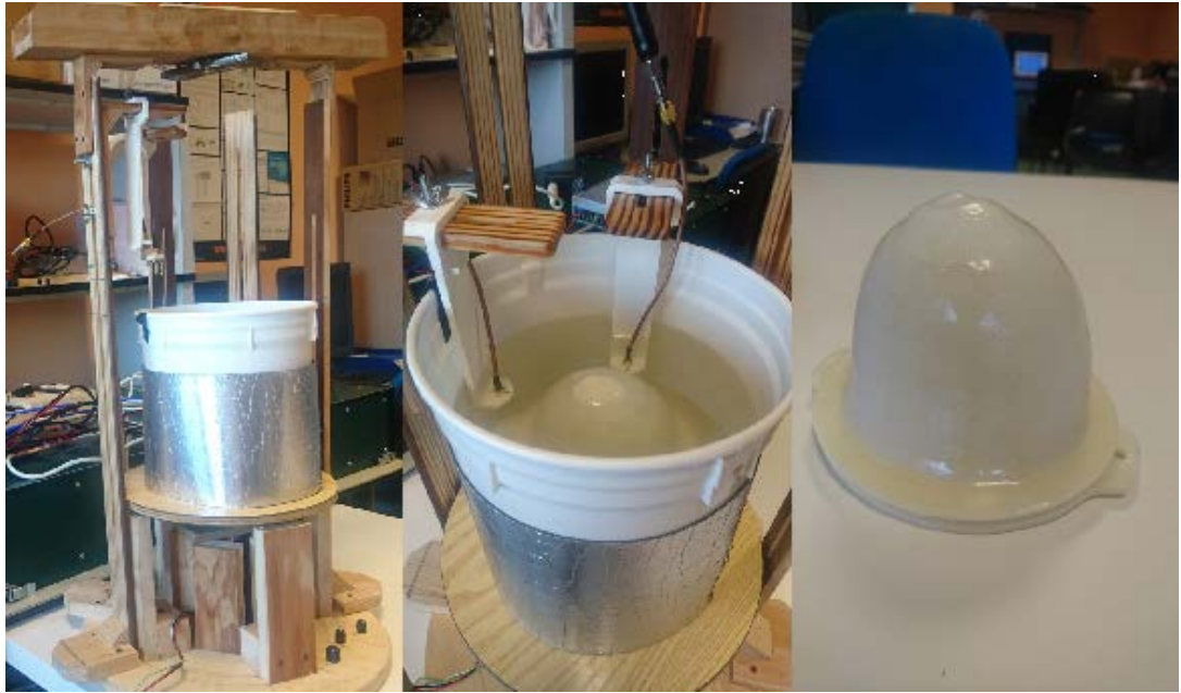
Figure 6.1: Set-up of the two-antenna experimental MWI system developed in Politecnico di Torino.
