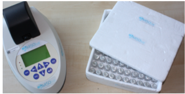
Portable luminometer used to quantify arsenic concentration in samples
