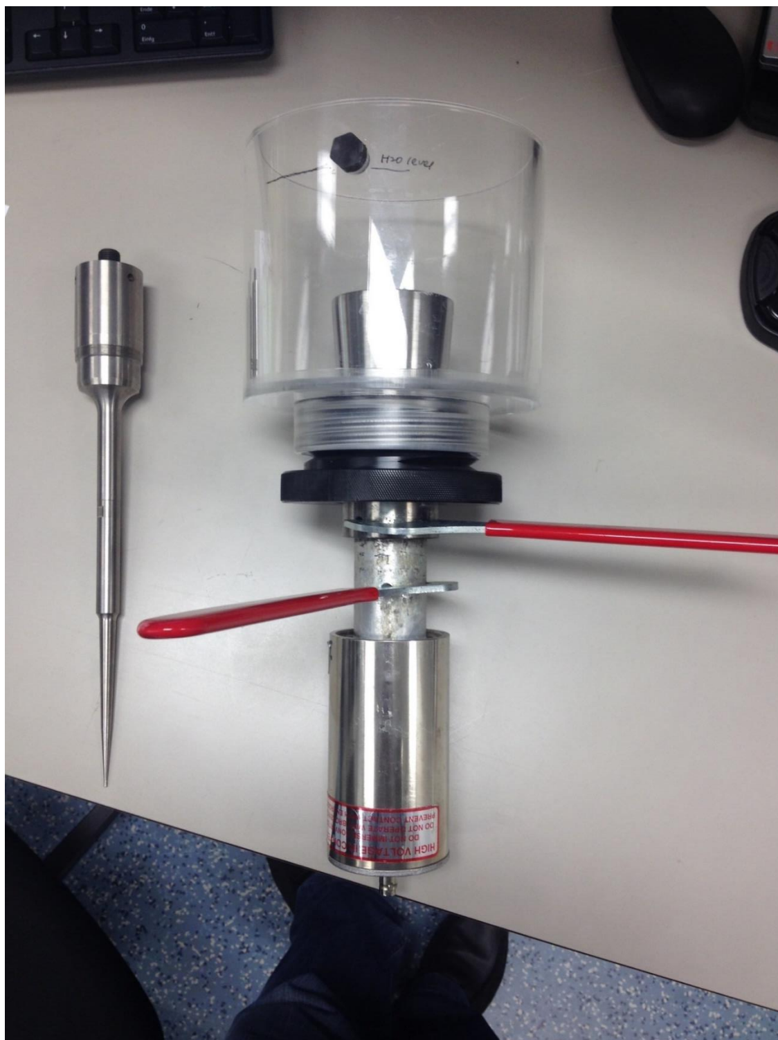
Figure 5.16: Setup for the S-4000 sonicator. The sonicator's tip (on the left) was removed and replaced with a 5'5 cuphorn (on the right) and a 20 kHz converter (underneath the cup horn).
